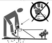
Do not push on the sensor housing or sprinkler head. If the ground is too hard or otherwise unsuitable for the plastic stake, order the CRO-200 Scarecrow Universal Mounting Bracket.
